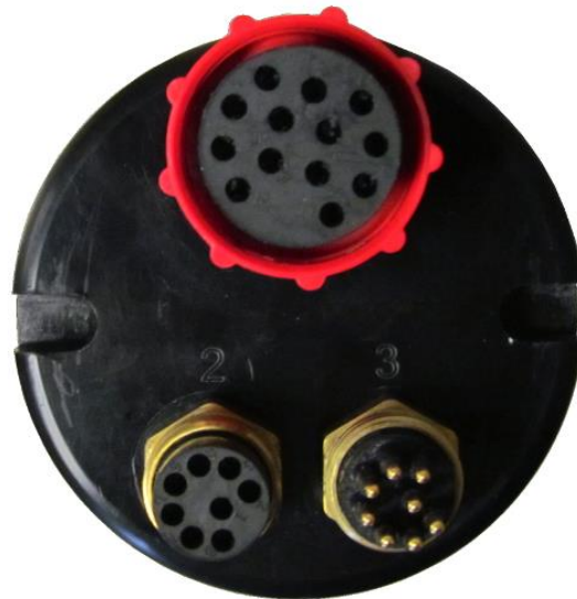
Figure 5-2: icLink with Bus Adapter, Uplink Ethernet and Serial Connectors
