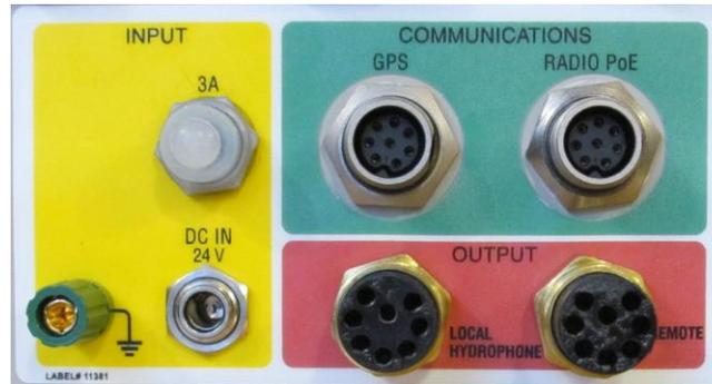
Figure 5-3: 48V Host Interface Operational Connectors
