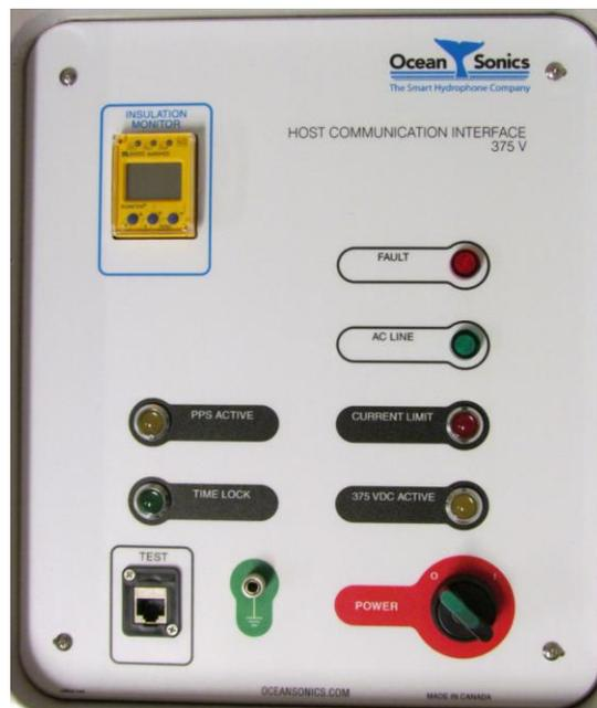
Figure 3-3: 375V Host Interface Internal Panel
