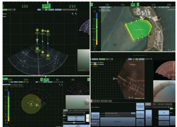
» Greensea's Workspace software already includes features like automated waypoint following, search grid and station keeping among others making it much easier to complete missions. (Image credit: Greensea)
