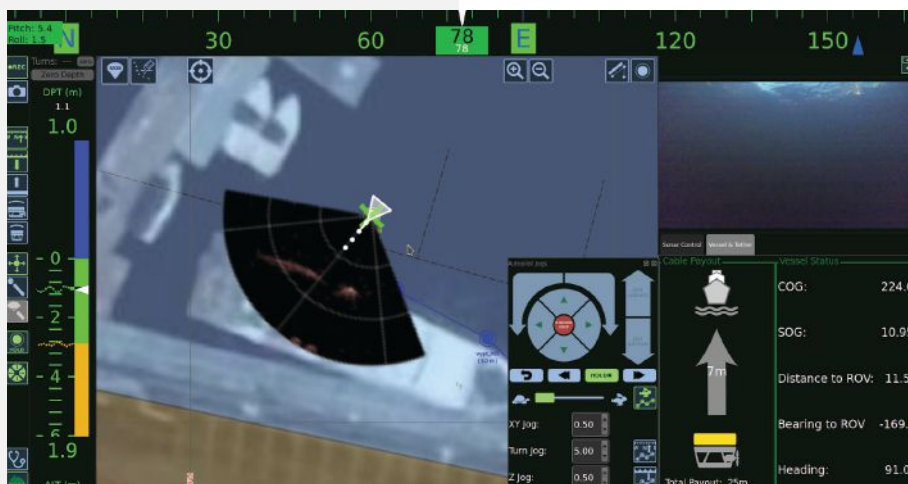
» EOD Workspace configuration with long range standoff module, vessel management module, and tether management module installed. (Image credit: Greensea)
