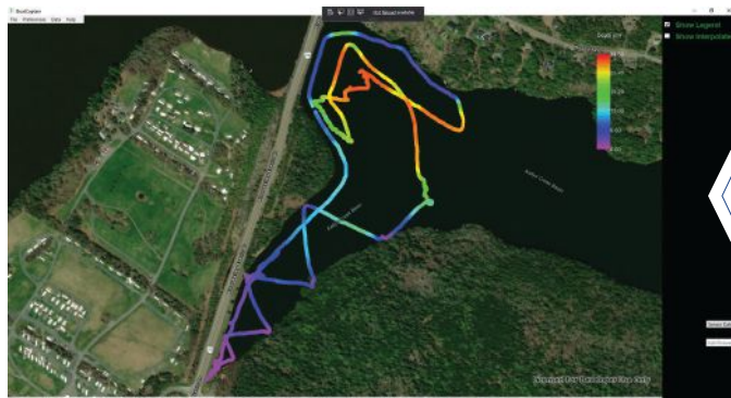
» A sample depth track obtained using a fish finder aboard AMOS. (In Nature Robotics)
