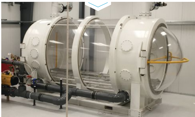
» Certified Acrylic Pressure Vessel for Subsea Habitat (Photo credit: Hydrospace Group)
