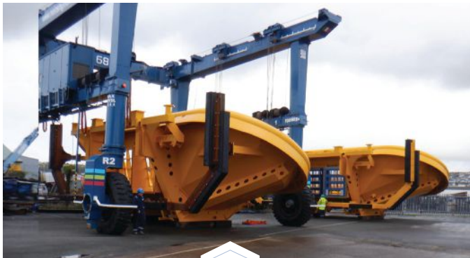
» Bombora's patented mWave™ is a unique modular system of flexible rubber membrane covered cell units, each 15 meters in length. (Photo credit: Bombora)
