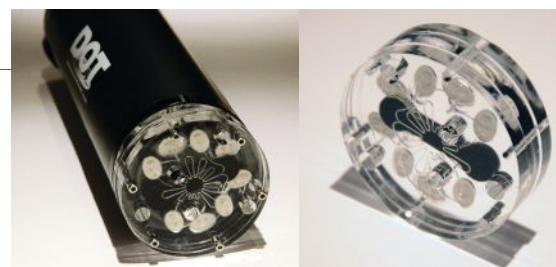
» Figure 2: An example lab-on-chip phosphate sensor. Patents pending. (Photo credit: Sieben Laboratory at Dalhousie University)
