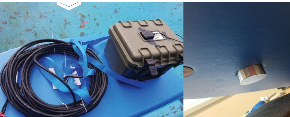
» A commercial single-beam echosounder (SBES) and a GPS evaluation kit mounted to a foam body board designed by the Department of Geodesy and Geomatics at HafenCity University (HCU) in Hamburg, Germany—an example of a low-cost multi sensor systems (MSSs) for hydrographic surveying. (Photo credit: Markus Kraft, HafenCity University Hamburg)
