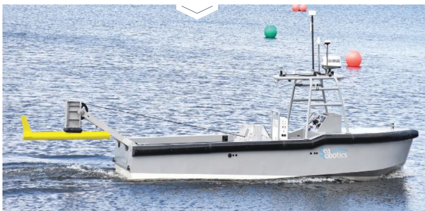
» SeaRobotics' SR-Endurance 7.0; multi-mission ASVs will become instrumental for defense and scientific applications. (Photo credit: SeaRobotics)
