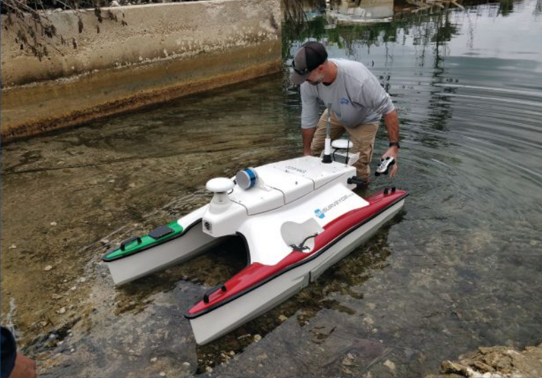
» The man-portability and plug-and-play capabilities of compact ASVs offer operators a key differential when it comes to survey efficiency. (Photo credit: M&E)
