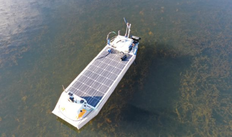
» In Nature Robotics' AMOS (Aquatic Mini Observation System), an autonomous, solar-powered airboat that is intended for long-term water quality monitoring and surveying applications. (Photo credit: In Nature Robotics)
