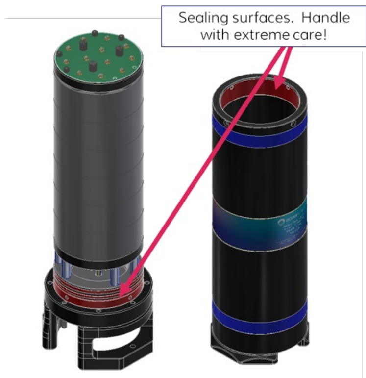
Figure 05: Battery pack sealing surfaces are shown in red
