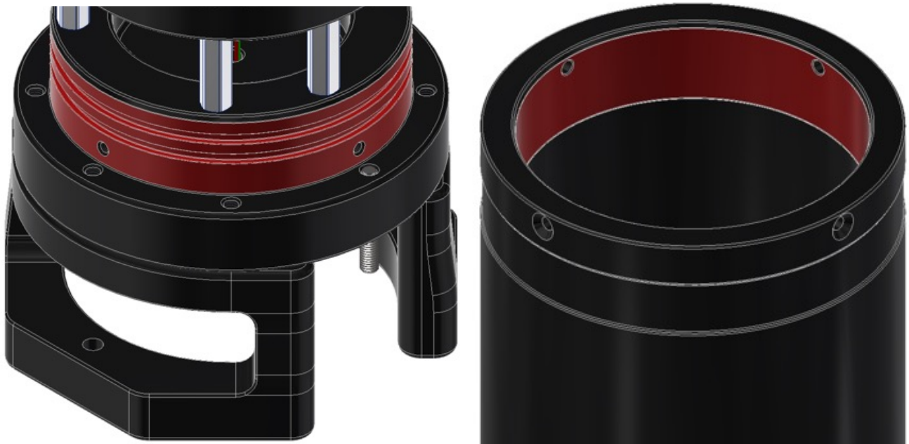
Figure 09: Sealing surface of the battery pack shown in red.
