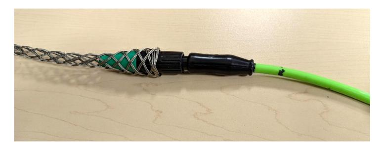
• Feed the connector through the cable grip and out the largest hole in the side.
