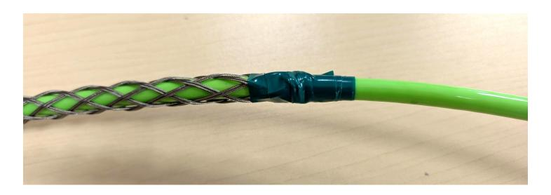
• The tape is **not** load bearing, it simply keeps the cable grip in position during handling, and begins the cascading radial tightening effect without any slippage.
