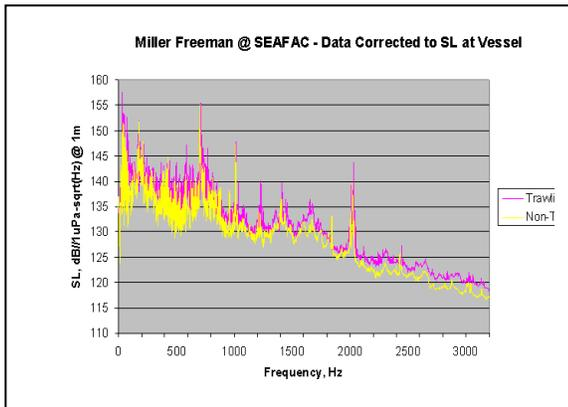
Fig. 5: Radiated-noise signature of a fishing vessel
