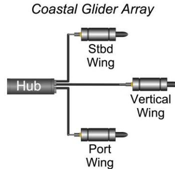
Fig. 3: Smart Hydrophone CG Array
