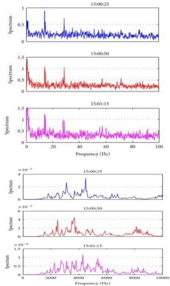
Fig. 2: Comparison of the full spectrum to the DEMON spectrum for a ferry.
