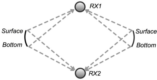
**Fig. 4: Ambiguity of a 2-hydrophone array**
