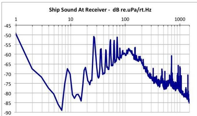
Fig. 6: Radiated noise signature of a cargo vessel.
