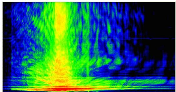
Fig. 4: Spectrogram: Passing of Small Vessel
