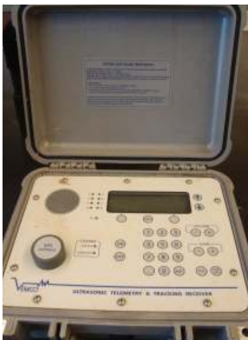
Figure 4. The VR100 manual tracking unit used to follow the Atlantic sturgeon bioprobe by picking up the V13P acoustic tag signal (ID 5711). It also picked up acoustic tag signals (IDs) from other tagged fish and provided a time and GPS location for each detection.
