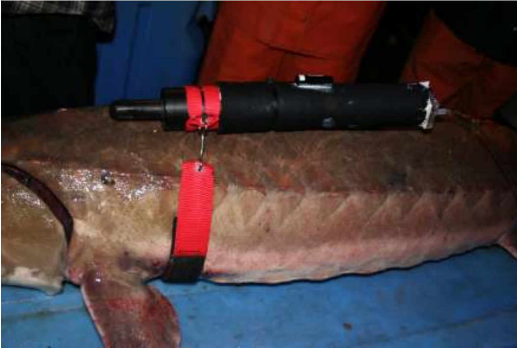
Figure 8. The complete icListen hydrophone “backpack” attached to the Atlantic sturgeon bioprobe and ready for deployment.
