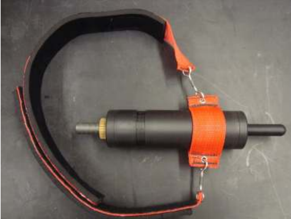
Figure 2. Velcro belt similar in design to the one used for the deployment of the icListen hydrophone on the Atlantic sturgeon. The nylon strap had industrial strength Velcro glued and sewn to it, as well as a layer of neoprene on the inside. In this image, the belt is loosely attached to a dummy hydrophone for testing purposes.
