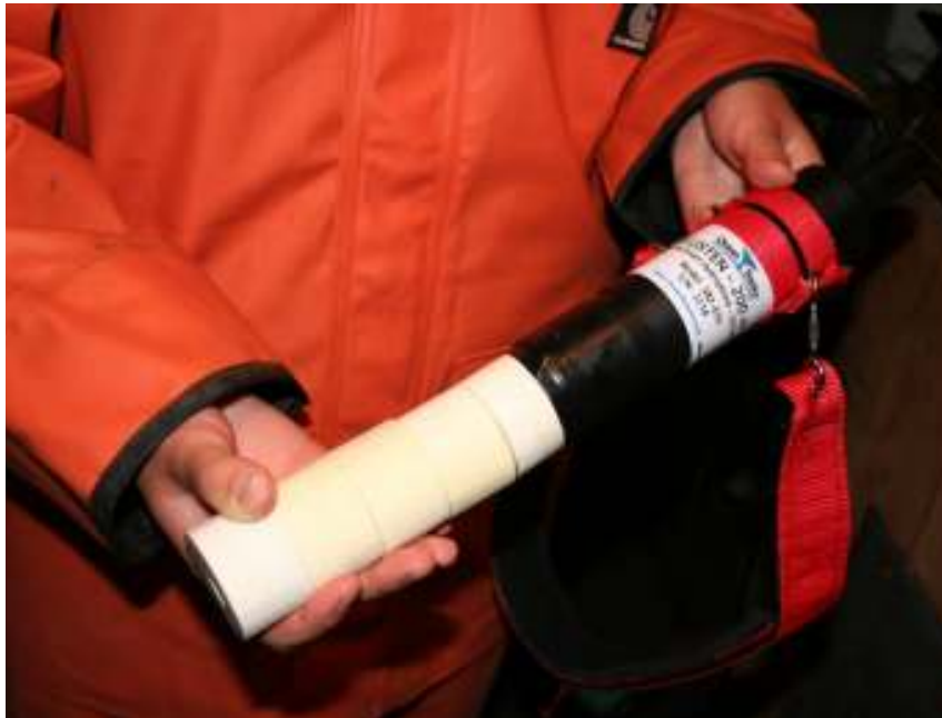
Figure 6. Five cylinders of syntactic foam glued together using a waterproof silicone and stacked onto the back end of the icListen hydrophone for flotation.
