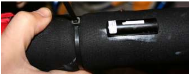
Figure 3. The V13P acoustic tag, glued to the exterior of the icListen , used to track the Atlantic sturgeon bioprobe during the deployment.
