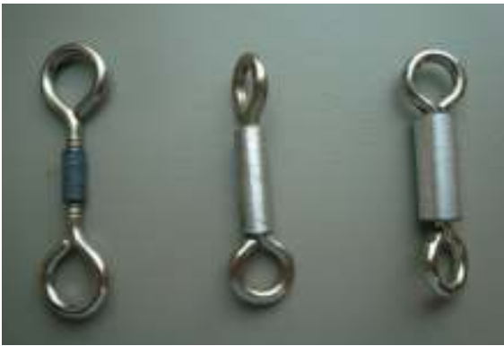
Figure 5. Three types of galvanic releases with different amounts of the metal alloy; the AA2 (6 hour) type, on the left, was used in the icListen hydrophone deployment.
